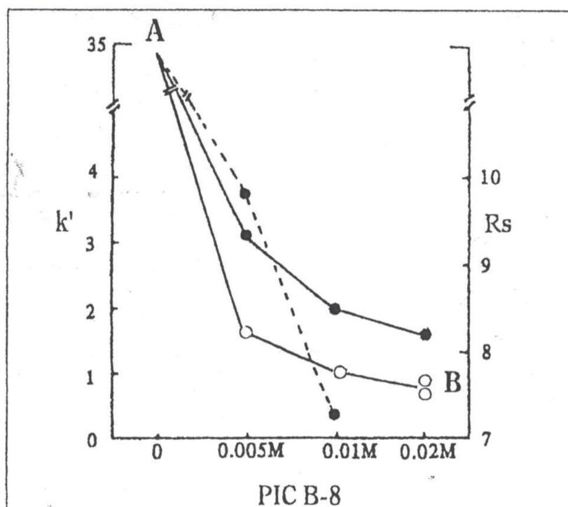
Figure 2. Effect of the concentration of PIC B-8 on the  $k'$  value of PYR (●—●) and OMT (○—○) and the  $R_s$  between them (●---●): (A) only solvent peaks before 70 min and (B) the peak of OMT split into two overlapped peaks when the concentration of PIC B-8 was 0.02M. All eluents were 60% acetonitrile in water overall.
