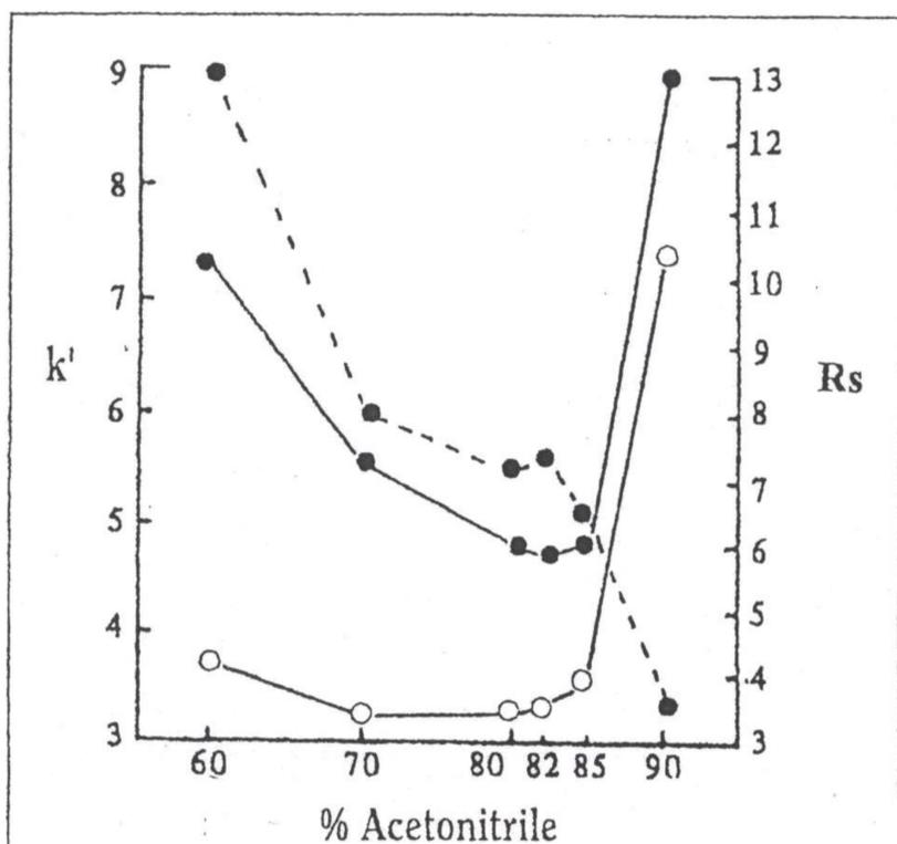
Figure 1. Effect of the proportion of acetonitrile on the  $k'$  value of PYR (●—●) and OMT (○—○) and the  $R_s$  between them (●---●). All eluents were acetonitrile in 0.005M PIC B-8 overall.
