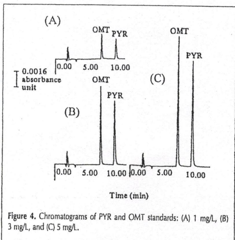
Figure 4. Chromatograms of PYR and OMT standards: (A) 1 mg/L, (B) 3 mg/L, and (C) 5 mg/L.
