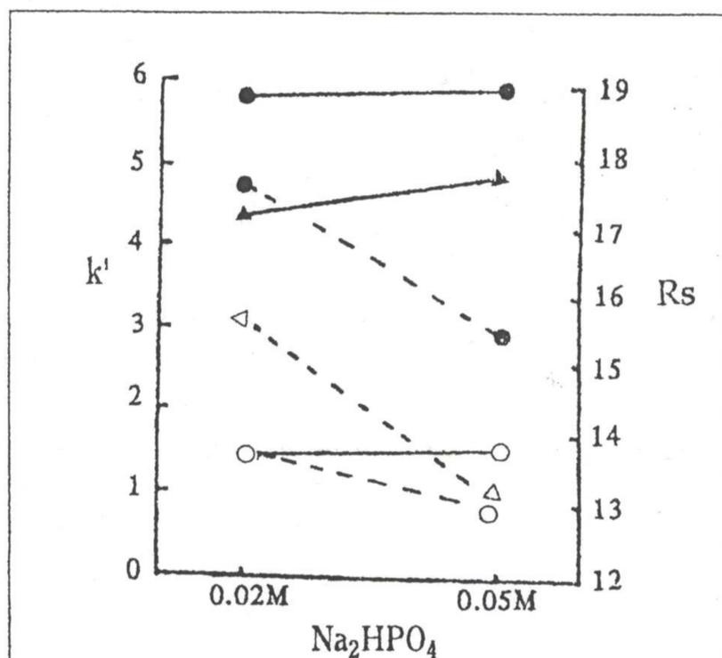
Figure 3. Effect of pH and the concentration of  $\text{Na}_2\text{HPO}_4$  on the  $k'$  value of PYR and OMT and the  $R_s$  between them: PYR at pH 7.5 (●—●), PYR at pH 4.0 (●---●), OMT at pH 7.5 (○—○), OMT at pH 4.0 (○---○),  $R_s$  at pH 4.0 (▲---▲). All eluents were 40% acetonitrile in water.
